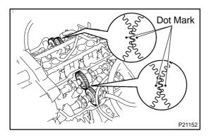
(b) Check that the timing marks (1 dot) of the camshaft drive and driven gears are in straight line on the cylinder heads surface as shown in the illustration.
