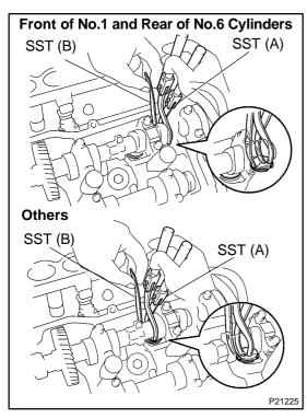
(3) Using SST (A), press down the valve lifter and place SST (B) between the camshaft and valve lifter. Remove SST (A).
