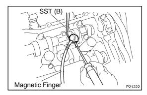
(4) Using a small screwdriver and magnetic finger, remove the adjusting shim.
