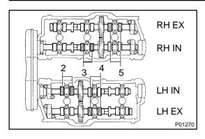
(b) Turn the crankshaft 2/3 of a revolution (240°), and check only the valves indicated in the illustration. Measure the valve clearance (See step (a)).
