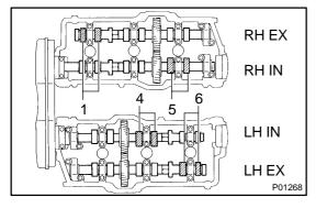
(c) Turn the crankshaft a further 2/3 of a revolution (240°), and check only the valves indicated in the illustration. Measure the valve clearance (See step (a)).
