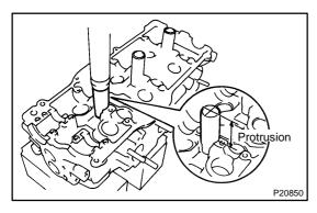
(b) Using a press, press in the spark plug tube until there is 49.0 – 49.4 mm (1.929 – 1.945 in.) protruding from the camshaft bearing cap installation surface of the cylinder head.
