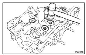
(d) Using a plastic–faced hammer, lightly tap the valve stem tip to ensure a proper fit.
